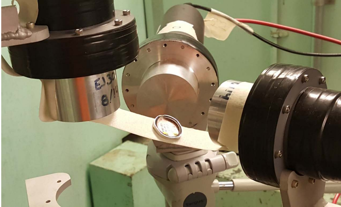
Figure 9. The three detectors arranged around a ^{60}\text{Co} for the calibration run 3 measurements.
